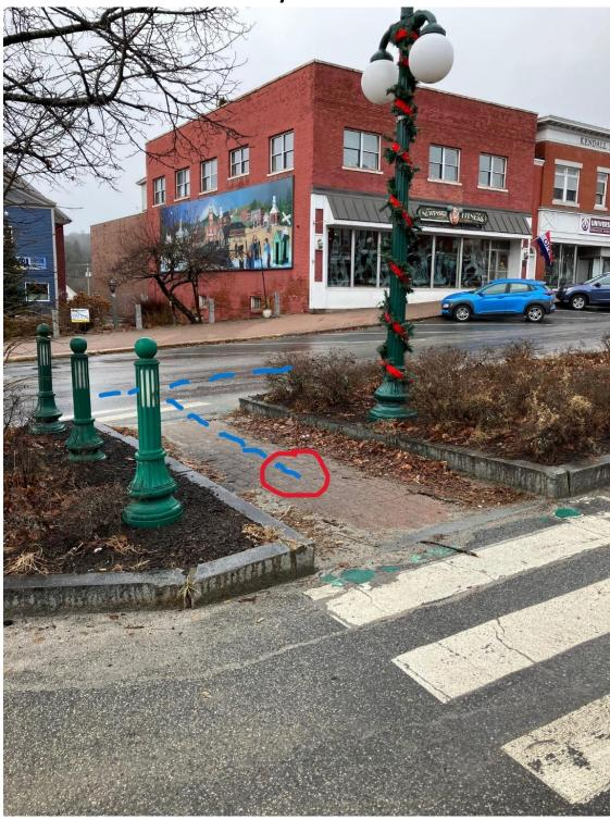
Connect new hydrant to existing 10" cast iron water main via a live "wet tap". Install approximately 20' of 6" cement lined ductile iron pipe and new hydrant (hydrant supplied by the Town). Contractor to supply thrust blocks. Hydrant to be installed at top of curb elevation, centered in the middle and the two islands are to be joined to make one continuous island. Crosswalk will be abandoned.
