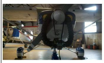
prior to flight. The AeroTherm heater is thermostat controlled and runs on electricity making it preferred over the use of kerosene or propane fired heaters. The heater is available free of charge for all, however donations are greatly appreciated.
