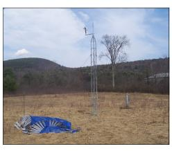
self-contained, solar powered unit that records wind speed and direction, temperature, and rainfall. The station is not an aviation weather station and although the information will be available on the web, it is not directly available to pilots for aeronautical purposes.
