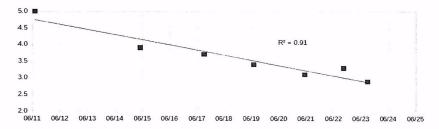
The current results show a continuing deterioration of the runway. This deterioration is a normal and expected condition in the pavement lifecycle. All pavements wear out and fail, eventually becoming hazardous, unsafe, and unsuitable for use by aircraft whether taxiing, taking off, or landing. As a baseline for comparison, the PASER index was 2.6 in 2010 before the runway was repayed in 2011.
