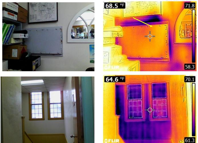
Lastly, there is the issue of the conductivity of the brick. Below are images of you and an employee, literally radiating your body heat to the glass and to the brick also highly conductive, uninsulated brick walls.
