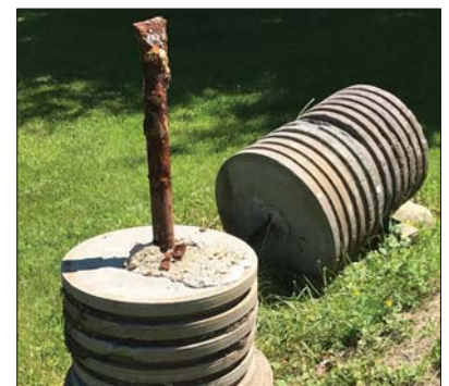
Castellated Grindstones (27 inch diameter)
