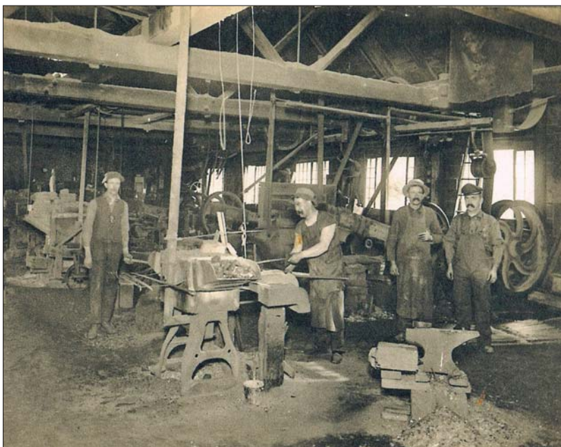
Scythe Shop - Note large trip hammer (diagonal beam)
